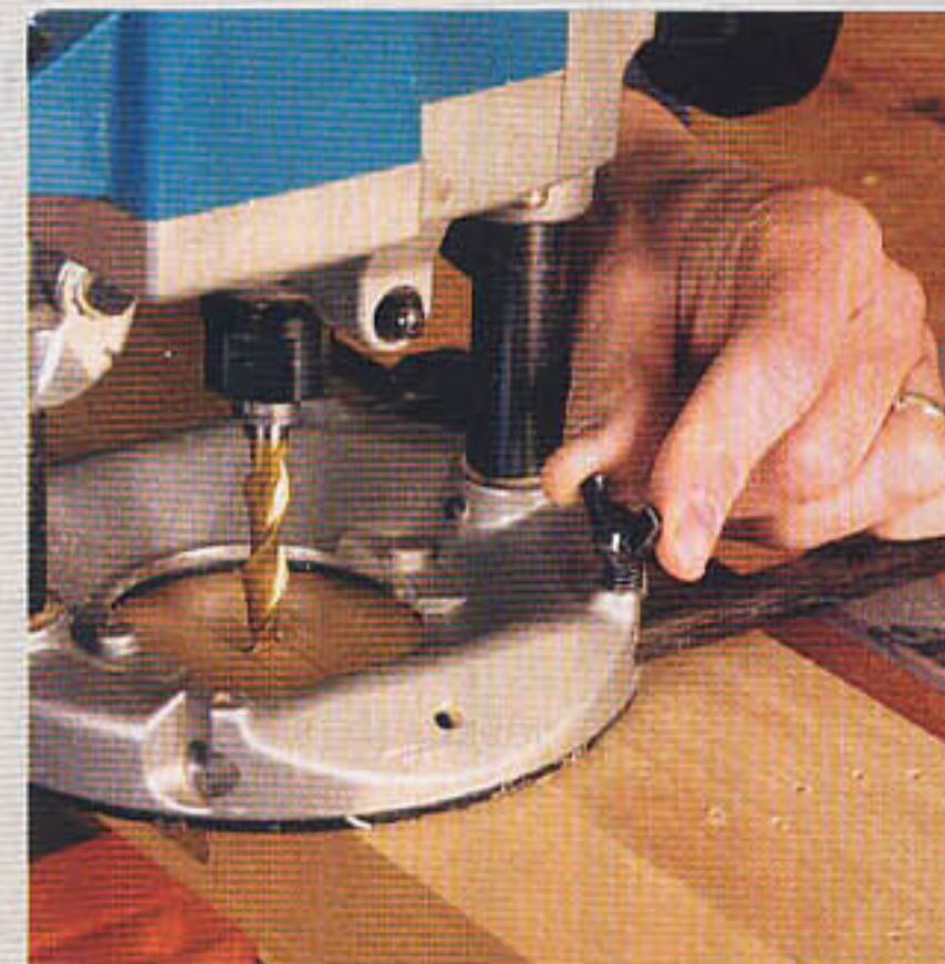
Center the bit. After marking the location of the mortise, adjust the edge guide to center the bit in the mortise.
