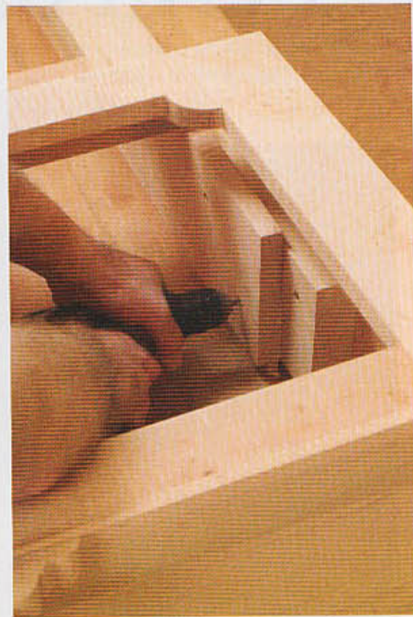
Attach the waist to the base. Where the waist sides extend down into the base cabinet, use plenty of glue and screws to secure the two cases to one another. Position them carefully before driving the screws through the waist sides into the glue blocks in the base. Once the glue sets, the waist and base become one cabinet. The bottom cove molding will conceal the gap between the two components.
