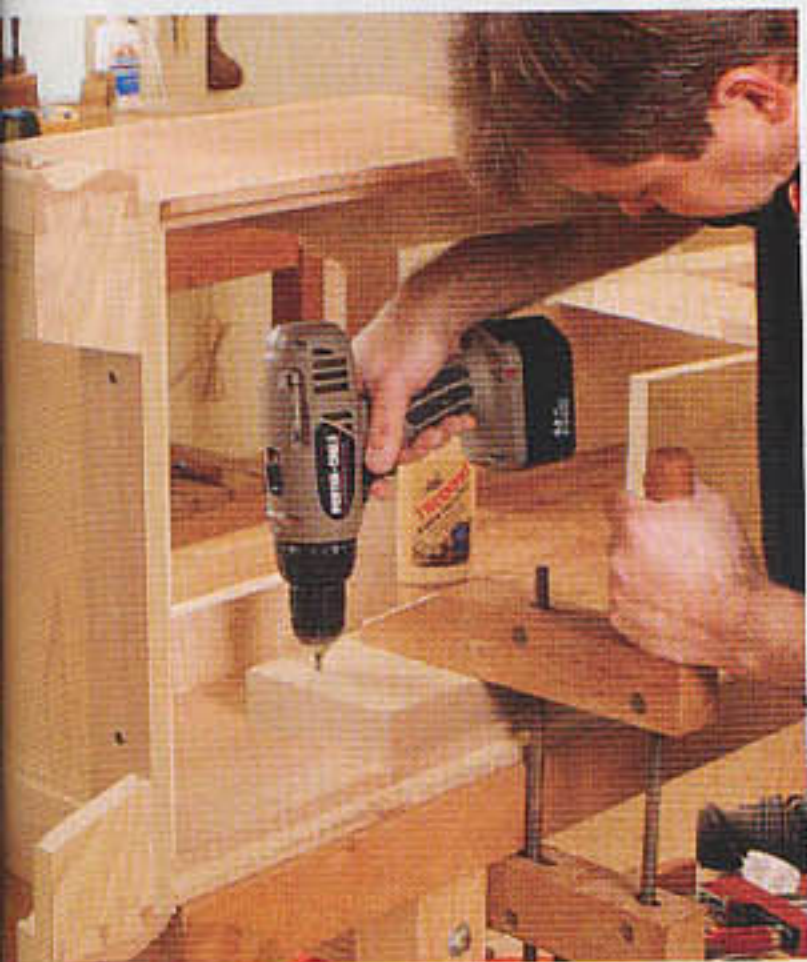
Glue blocks join the waist to the base. After assembling the waist and the base cabinets, measure the outside width of the waist and the inside width of the base. The difference divided by two is the thickness at which you should mill each of the two glue blocks. Glue and screw the blocks to the insides of the base cabinet first.
